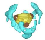
Nuclear scattering density map of CH<sub>3</sub>NH<sub>3</sub> molecule as derived from the Maximum Entropy Method showing C and N (yellow) and hydrogen scattering (blue)
