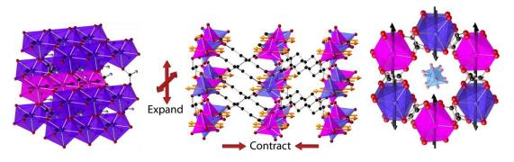
Figure: Structure of left) Magnetocaloric  $Tb(HCO_2)_3$  featuring 1D ferromagnetic chains packed in an antiferromagnetic triangular lattice, middle) Co(adipate) which shrinks in one dimension as it magnetically orders due to its anisotropic magnetic coupling and right) multiferroic NH<sub>4</sub>Co(HCO<sub>2</sub>)<sub>3</sub>, which has ferroelectric properties across a broad temperature range.
